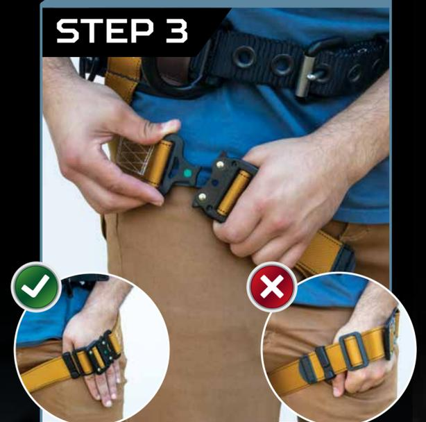
Pull leg straps up and between legs then connect to buckles located closest to each hip.
