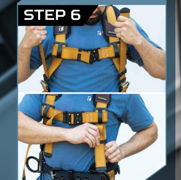
While standing up straight, adjust torso straps to your height and to remove slack.
