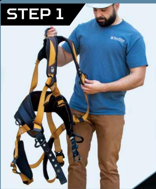
Holding the harness by the dorsal D-ring, shake it to allow all straps to hang freely and untwisted.
